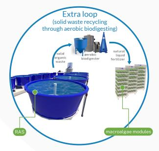
**Gloasis** has developed a highly productive vertical modular macroalgae system, which gets the input of  $CO_2$ -rich air from the Recirculating Aquaculture System (RAS) unit (fish and bacteria), speeding up the growth of macroalgae and  $CO_2$  capture.
